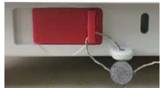
Locked with Wire Seal
